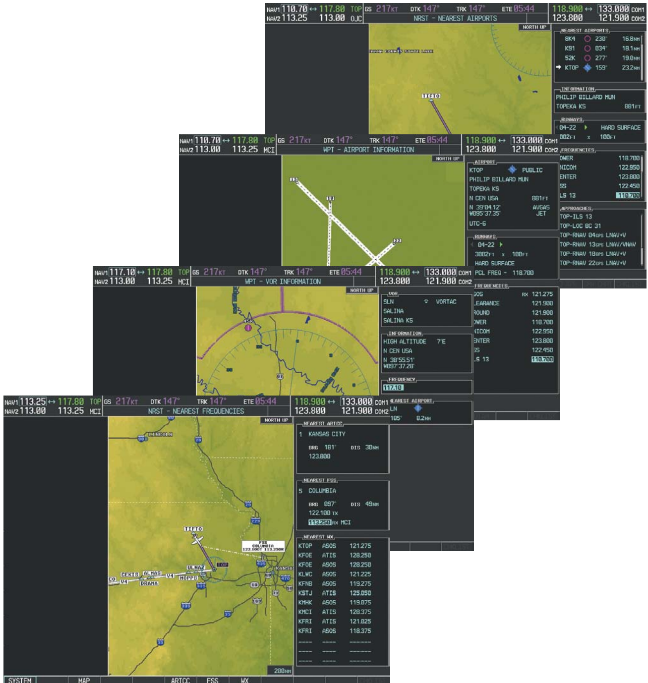
Figure 4-26 NRST – Nearest Frequencies, WPT – VOR Information, WPT – Airport Information, and NRST – Nearest Airports Pages
